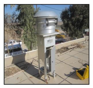
Figure 4: Hi-volume air sampler
