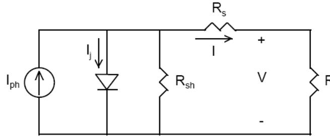
**Figure 1:** Equivalent circuit for solar cell.
